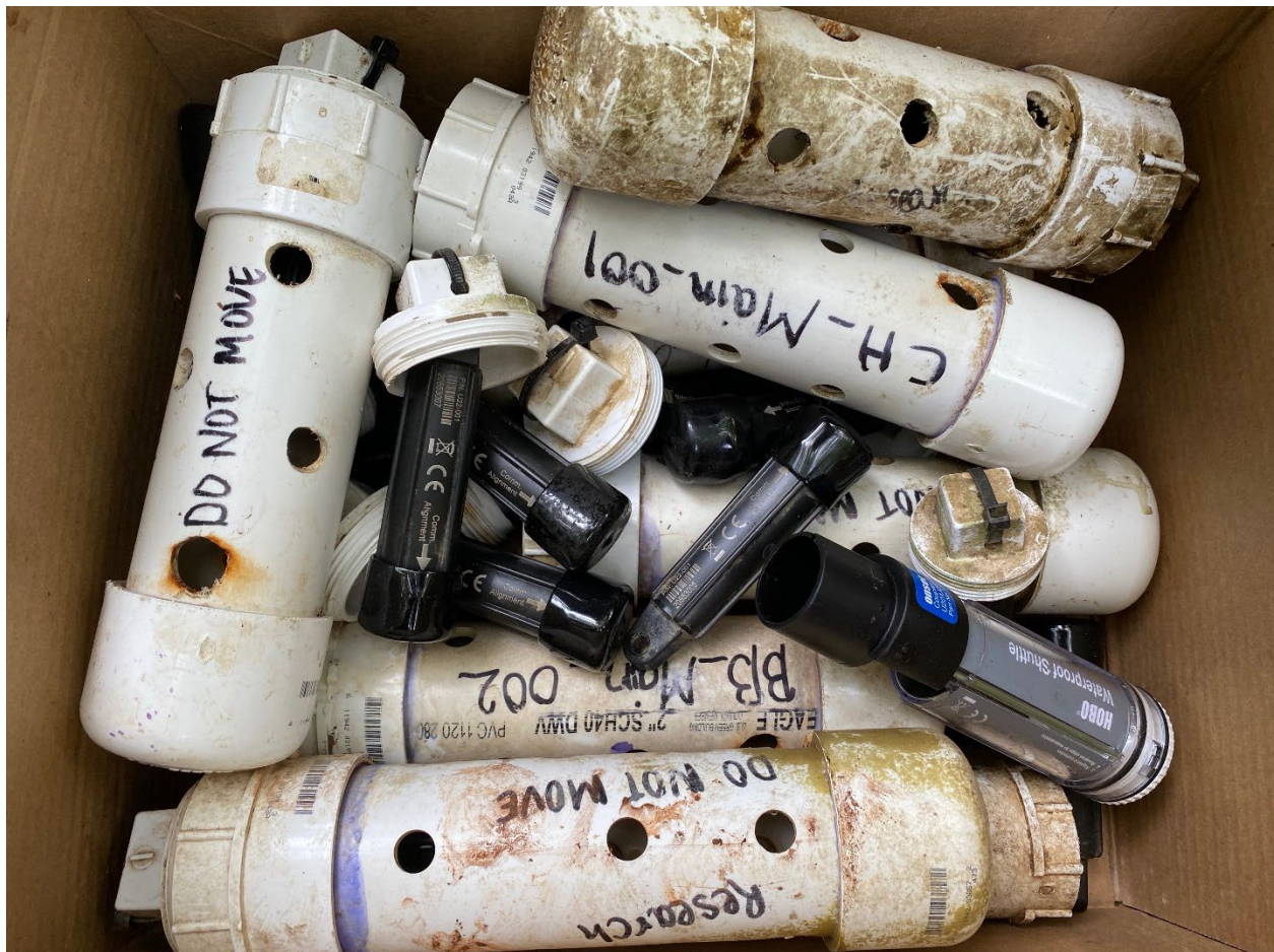
Above: Temperature monitoring equipment. HOBO Data Loggers, protective PVC housing, and data offload shuttle.
